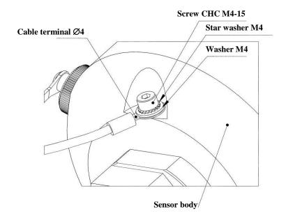
The earth connection must be realized according to the rules of conduct, by qualified personnel.
