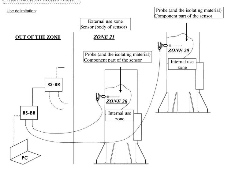
The trib'atex-SPX50 are connected to RS-BR interface units.
