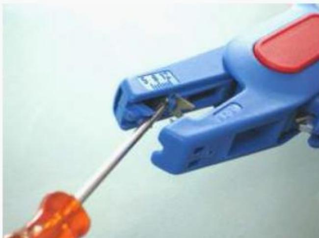
Press the handles of the plier together and release it slightly so that the fixing screw of the upper blade appears. Open the screw with a crosstip screw driver and remove the blade. Insert the new blade facing the sharp side downwards and fix it again with the screw.
