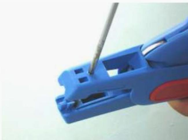
Remove the lower blade by pressing it out of its guide with a screw driver through the hole in the lower jaw. Insert the new blade facing the sharp side upwards and press it back gently into its guide. Insert the adjustable length stop back into the guide rail.
